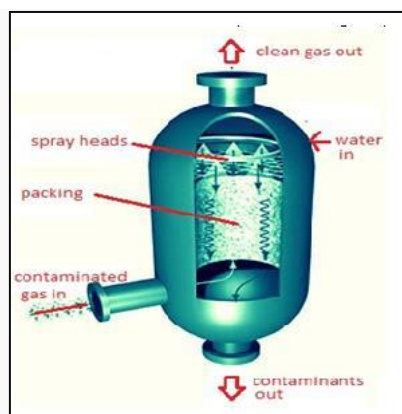
Fig. a scrubber
